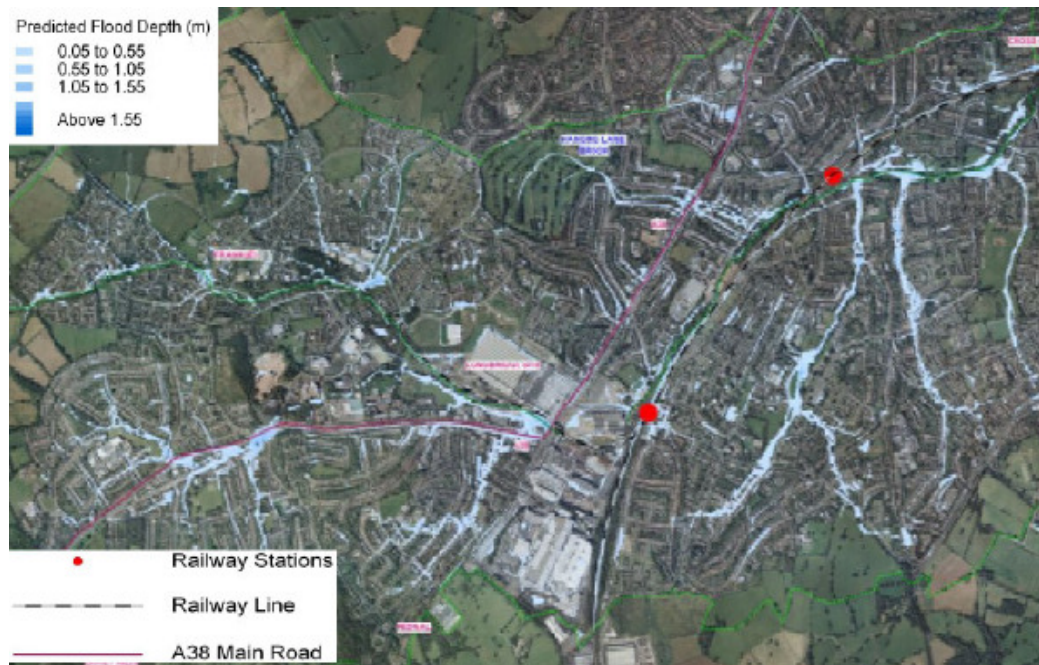
Figure 6 Predicted 1:100 RI Surface Flooding for the Upper Rea, Birmingham. (From: Birmingham City Council, 2008)
