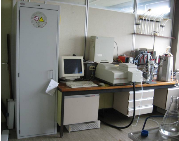
Figure 7.6: Experimental set-up for oxidation of liquid medium (water, urine) with ozone (oxygen bottle in the closet, computer for data reading, spectrophotometer for O 3 concentration, reactor, ozone generator (at the end, white box not to see), mass flow meter (also not shown)).
