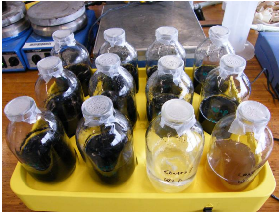
Figure 7.2: Flasks containing urine or water, different types of GAC and the same concentrations of pharmaceuticals.
